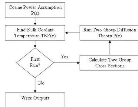
Figure -1: The in-house thermal hydraulic program flow chart.
