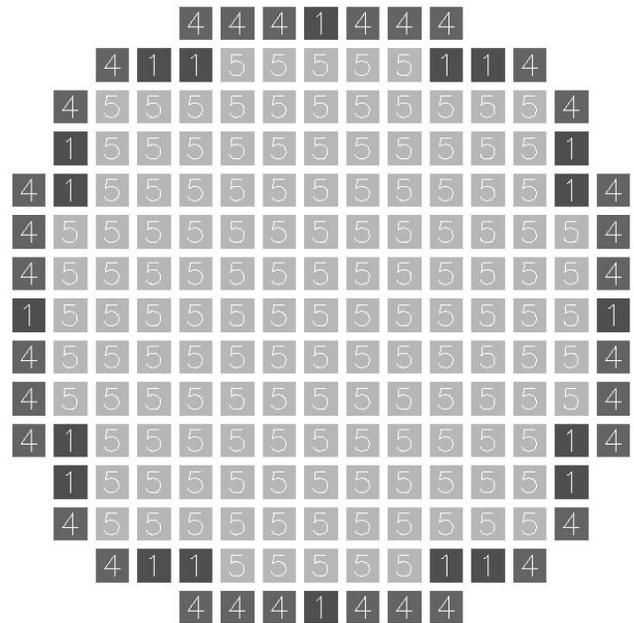
Figure -9: Core loading pattern for the bottom axial zone (25”).
