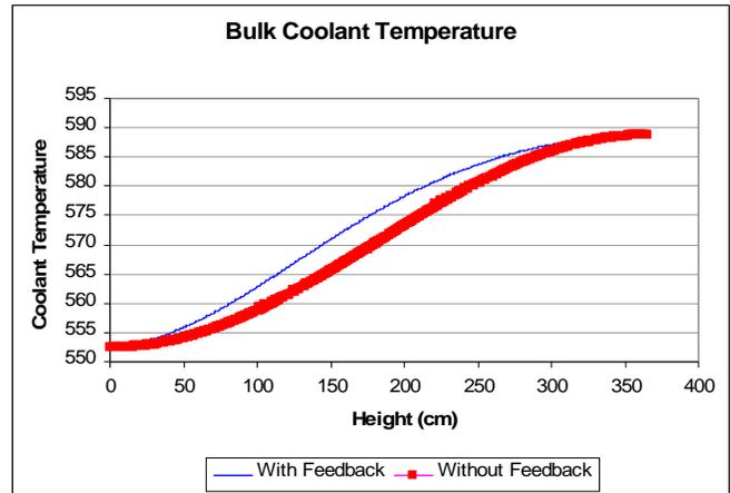
Figure -24: Bulk coolant temperature for the PRATT fuel design in Kelvin as a function of core height.
