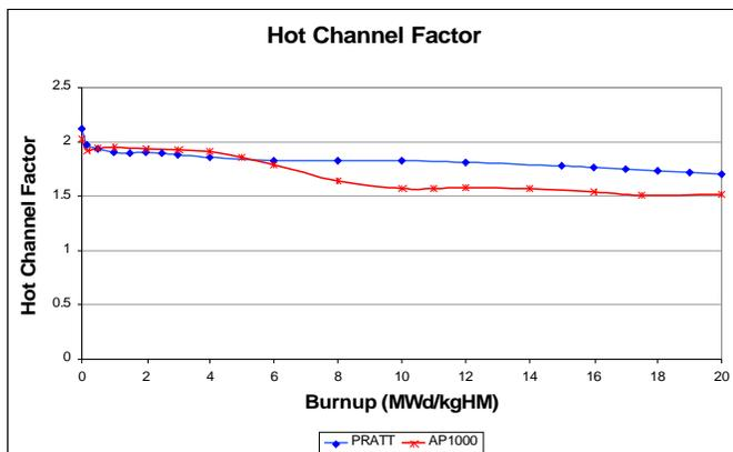
Figure -16: Maximum overall hot channel factor,  $F_{q,}$  as a function of burnup in MWd/kgHM comparing the PRATT fuel design with the AP1000.
