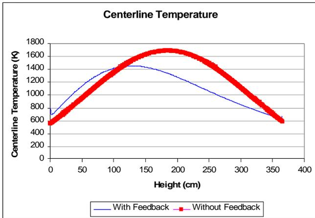
Figure -26: The fuel centerline temperature in units of Kelvin as a function of core height from bottom for both the AP1000 and PRATT fuel designs.
