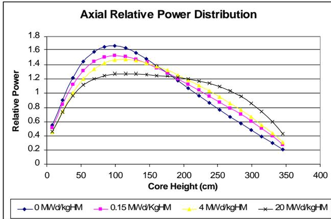
Figure -19: The PRATT axial relative power distribution before axial zoning.
