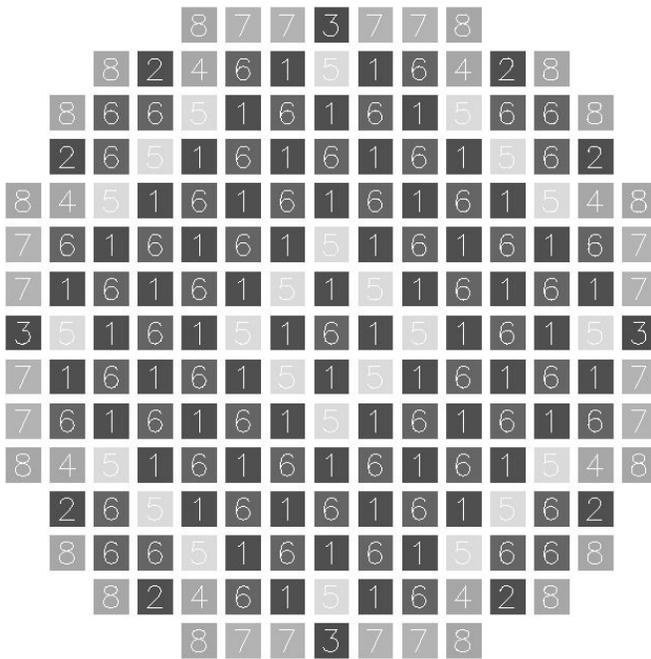
Figure -8: Core loading pattern for the central axial zone showing the placement of the 193 assemblies.
