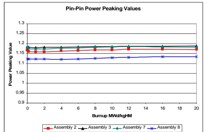
Figure -14: Pin to pin power peaking values for the higher enriched assemblies (2, 3, 7, 8) as a function of burnup MWd/kgHM.
