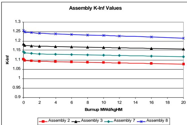
Figure -12: K-inf values for the four higher enriched assemblies (2, 3, 7, 8) as a function of burnup in MWd/kgHM
