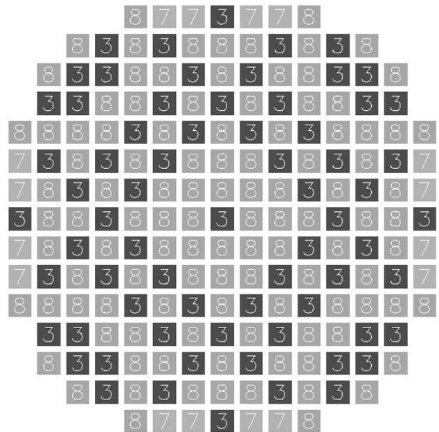
Figure -10: Core loading pattern for the top axial zone (15”).
