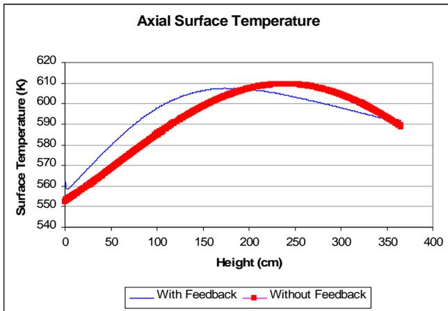
Figure -25: PRATT and AP1000 fuel surface temperature in Kelvin as a function of core height.
