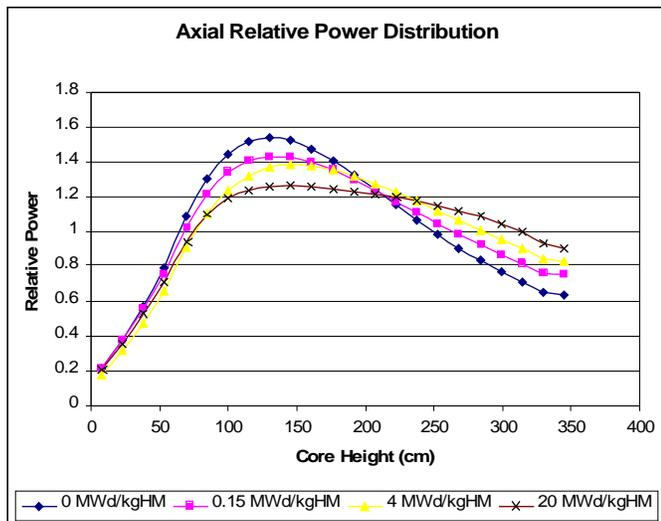
Figure -20: The axial relative power distribution of the PRATT fuel design at four different burnups.
