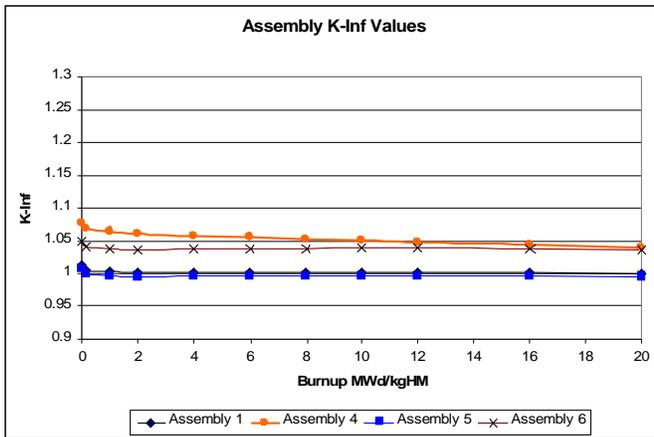
Figure -11: K-inf values for the four lower enriched assemblies (1, 4, 5, 6) as a function of burnup in MWd/kgHM.
