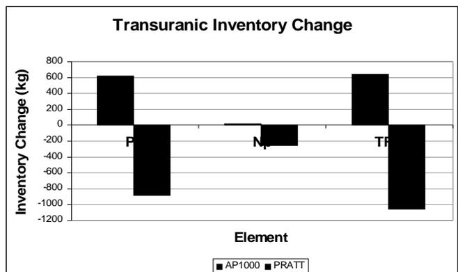
Figure -22: Transuranic inventory changes over one cycle length for the PRATT fuel and AP1000 design.
