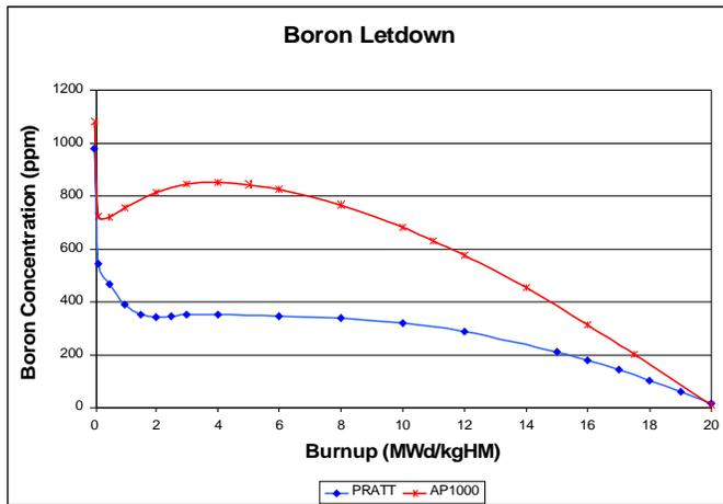
Figure -15: Boron concentration as a function of burnup, MWd/kgHM, comparing the PRATT and AP1000 designs.
