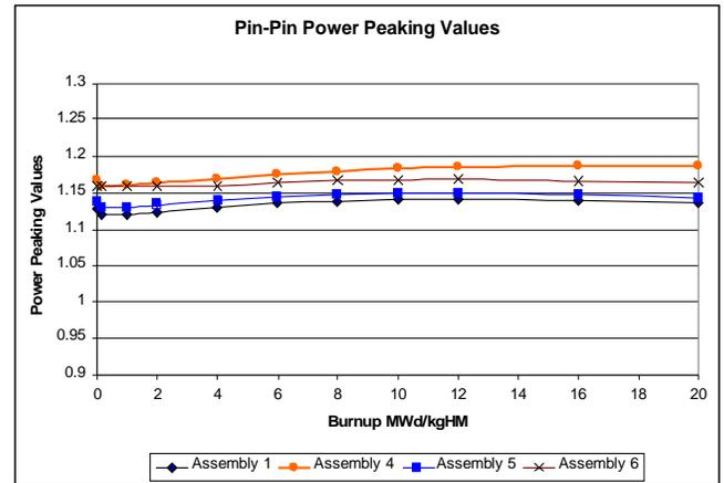
Figure -13: Pin to pin power peaking values for the low enriched assemblies (1, 4, 5, 6) as a function of burnup MWd/kgHM.
