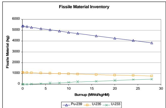
Figure -21: Fissile isotope inventory in kg as a function of burnup MWd/kgHM.
